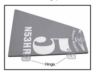
□ 3) Slide the rudder on the fuselage panel until there is only a slight gap. The hinge is now centered on the fuselage panel and rudder. Remove the T-pins and snug the rudder against the fuselage panel. A gap of 1/64" or less should be maintained between the fuselage panel and rudder.
