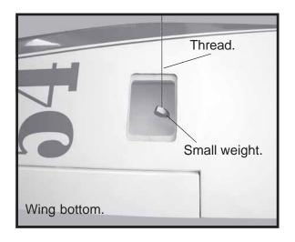
Attach servo lead to the aileron servo. Attach the string to the servo lead and carefully thread it though the wing. Once you have thread the lead throught the wing, remove the string so it can use for the other servo lead. Tape the servo lead to the wing to prevent it from falling back into the wing.
