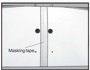
☐ 3) Peel off the backing from the self adhesive covering strip. Apply the strip to the centre section of the wing starting from the bottom trailing edge. Wrap the strip all the way around the wing until it meets the trailing edge again. Trim off any excess strip.
