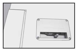
Install the aileron servo tray into the servo mount.
