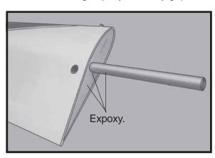
Carefully slide the two wing halves together and firmly press them together, allowing the excess epoxy to run out. There should not be any gap in the wing halves. Use rubbing alcohol and a paper tower to clean up any excess epoxy.
