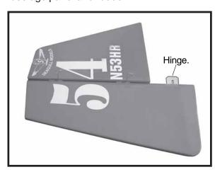
☐ 4)Deflect the rudder and completely saturate each hinge with thin C/A glue. The rudder front surface should lightly contact the fuselage during this procedure. Ideally, when the hinges are glued in place, a 1/64" gap or less will be maintained throughout the lengh of the rudder to the fuselage panel hinge line.
