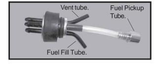
When the stopper assembly is installed in the tank, the top of the vent tube should rest just below the top surface of the tank. It should not touch the top of the tank.
