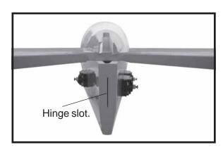
□ 2) Slide the vertical stabilizer into the slot in the top of the fuselage. The rear edge of the stabilizer should be flush with the rear edge of the fuselage and the lower rudder hinge should engage the precut hinge slot in the lower fuselage. The bottom edge of the stabilizer should also be firmly pushed against the top of the horizontal stabilizer.
