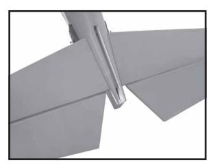
☐ 8) After the epoxy has fully cured, remove the masking tape or T-pins used to hold the stabilizer in place. Carefully inspect the glue joints. Use more epoxy to fill in any gaps that may exist that were not filled previously and clean up the excess using a paper towel and rubbing alcohol.
