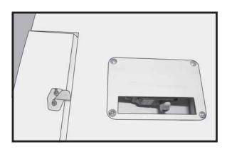
☐ 6) Thread one nylon adjustable control horn onto each aileron control rod. Thread the horns on until they are flush with the ends of the control rods.
