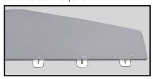
□ 3) Slide the elevator on the horizontal stabilizer panel until there is only a slight gap. The hinge is now centered on the horizontal stabilizer panel and elevator. Remove the T-pins and snug the elevator against the horizontal stabilizer panel. A gap of 1/64" or less should be maintained between the horizontal stabilizer panel and elevator.
