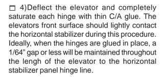
**Note:** The hinge is constructed of a special material that allows the C/A to wick or penetrate and distribute throughout the hinge, securely bonding it to the wood structure of the horizontal stabilizer panel and elevator.
