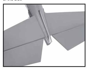
☐ 4) With the stabilizer held firmly in place, use a pen and draw lines onto the stabilizer where it and the fuselage sides meet. Do this on both the right and left sides and top and bottom of the stabilizer.
