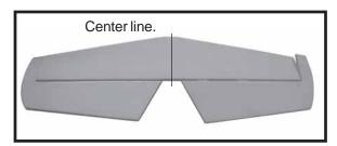
☐ 2)Using a modeling knife, carefully remove the covering at mounting slot of horizontal stabilizer ( both side of fuselage).
