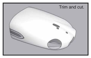
□2) While keeping the back edge of the cowl flush with the marks, align the front of the cowl with the crankshaft of the engine. The front of the cowl should be positioned so the crankshaft is in **nearly** the middle of the cowl opening. Use the spinner backplate as a guide. Hold the cowl firmly in place using pieces of masking tape.
