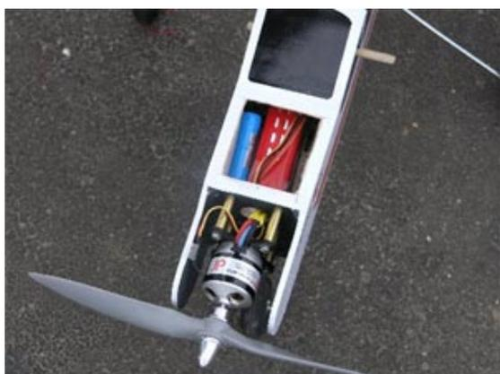
Ready to go. This photo (left) shows the hatch open shows some of the layout. Taped beside the motor is the RPM sensor of the datalogger. The LiPo is the red block seen through the hatch, the blue block is the 6v Rx battery. On the other side of the LiPo is the Opto ESC.
