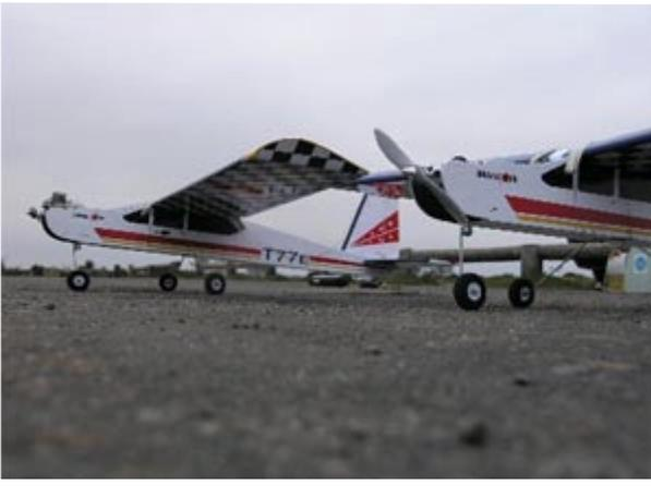
(Photo on the left. You're not seeing double! Electric in the foreground, .40 glow behind. Note the bent nose wheel leg of the glow model after 15 flights. It also felt greasy!)
