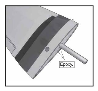
Carefully slide the two wing halves together and firmly press them together, allowing the excess epoxy to run out. There should not be any gap in the wing halves. Use rubbing alcohol and a paper tower to clean up any excess epoxy.
