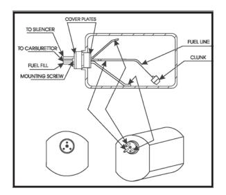
Slide the tank into the fuselage from inside so that the neck is at the top of the fuselage and it locates through the engine bulkhead. Gently secure it to the top horizontal former with the cable tie .
