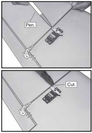
$\Box$  7) Make a 90-degree bend at the mark and cut off the excess wire leaving 7mm past the bend.
