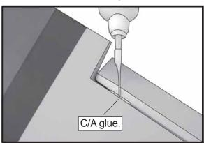
$\Box$  5) Turn the wing panel over and deflect the aileron in the opposite direction from the opposite side. Apply thin C/A glue to each hinge, making sure that the C/A penetrates into both the aileron and wing panel.
