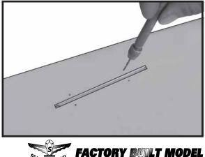
5) Remove the two straps and the gear wire. Drill four 1mm pilot holes into the wing for the wood screws.
