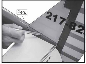
□ 4) Remove the stabilizer. Using a modelling knife, remove the covering from below the lines you drew. Also remove the covering from the bottom edge of the stabilizer and the bottom and top edges of the filler block. Leave the covering in place on the sides of the filler block.
