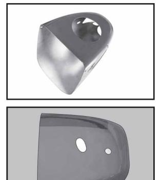
□ 2) Slide the fiberglass cowl over the engine and line up the back edge of the cowl with the marks you made on the fuselage.
