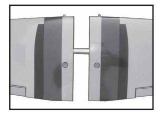
□ 3) Peel off the backing from the self adhesive covering strip. Apply the strip to the centre section of the wing starting from the bottom trailing edge. Wrap the strip all the way around the wing until it meets the trailing edge again. Trim off any excess strip.
