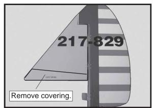
□ 5) Slide the vertical stabilizer back in place. Using a triangle, check to ensure that the vertical stabilizer is aligned 90° to the horizontal stabilizer.
