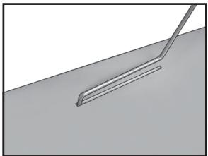
□ 3) The landing gear wire is held in place using two nylon landing gear straps and four 3mm x 10mm wood screws.
