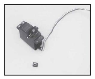
□ 2) Temporarilly install the aileron servo into the servo mount, with the output shaft towards the leading edge of the wing. Drill 1mm pilot holes through the mount. Remove the servo from the wing.
