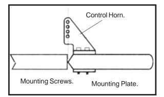
$\Box$ 3) Using a 1.5mm drill bit and the control horns as a guide, drill the mounting holes through the elevator halves.
