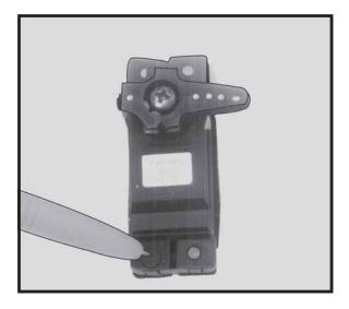
□ 3) Tie a weight such as the fuel tank pickup to a piece of string. Carefully feed the string through the wing and out of the servo.
