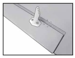
$\Box$  6) With the aileron servo centered and the aileron even with the trailing edge of the wing attach the clevis to the control horn. Mark the control wire where it crosses the servo arm hole.
