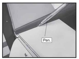
□ 2) Remove the stabilizer. Using the lines you just drew as a guide, carefully remove the covering from between them using a modeling knife.
