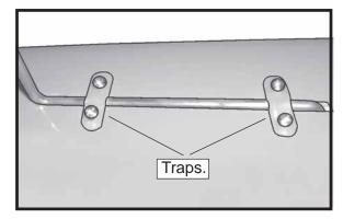
□ 6) Reinstall the gear wire and install the straps using the four 3mm x 10mm wood screws. Tighten the screws completely to secure the gear wire in place.
