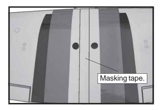
□ 4) When the epoxy has cured, carefully remove the masking tape from the wing.
