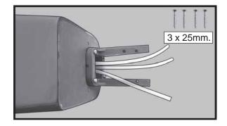
□ 1) Install the pushrod housing through the predrilled hole in the firewall and into the servo compartment. The pushrod housing should protrude 1/4" out past the front of the firewall. Make a Z-Bend 1/4" from one end of the plain wire pushrod.
