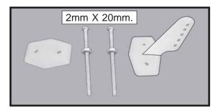
□ 3) Position the aileron horn on the bottom side of aileron. The clevis attachment holes should be positioned over the hinge line.
