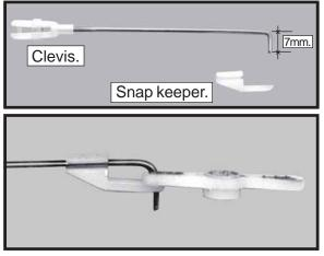
□ 9) Connect the linkage as shown and secure the control wire with a wire keeper.
