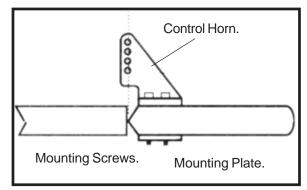
$\Box$  4)Using a 1mm drill bit and the control horns as a guide, drill the mounting holes through the aileron halves.
