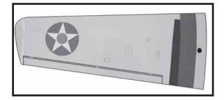
Note: <u>Work the aileron up and down several</u> <u>times to "work in" the hinges and check</u> for proper movement.
