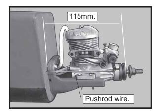
□ 2) Bolt the engine to the engine mount using the four machine screws.
