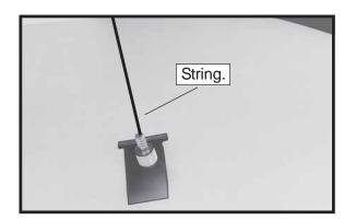
$\Box$  4) Attach the string to the servo lead and carefully thread it though the wing. Once you have thread the lead throught the wing, remove the string so it can use for the other servo lead. Tape the servo lead to the wing to prevent it from falling back into the wing.
