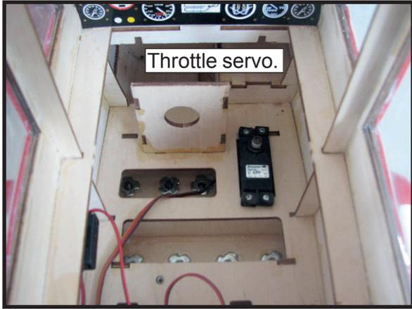
**THROTTLE SERVO ARM INSTALLATION.**
