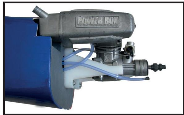
**!** Blow through one of the lines to ensure the fuel lines have not become kinked inside the fuel tank compartment. Air should flow through easily.
