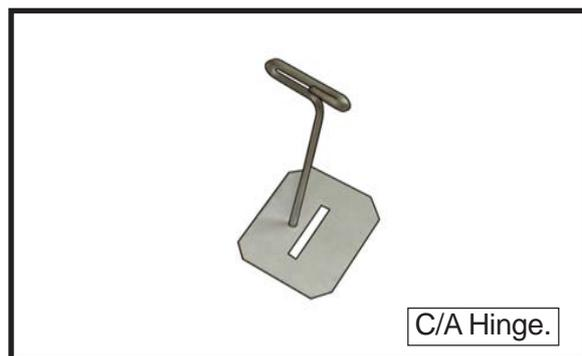
□ 2) Remove each hinge from the wing panel and aileron and place a T-pin in the center of each hinge. Slide each hinge into the aileron until the T-pin is snug against the aileron. This will help ensure an equal amount of hinge is on either side of the hinge line when the aileron is mounted to the wing panel.
