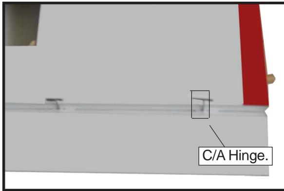
□ 4) Deflect the flap and completely saturate each hinge with thin C/A glue. The ailerons front surface should lightly contact the wing during this procedure. Ideally, when the hinges are glued in place, a 1/64" gap or less will be maintained throughout the length of the flap to the wing panel hinge line.
