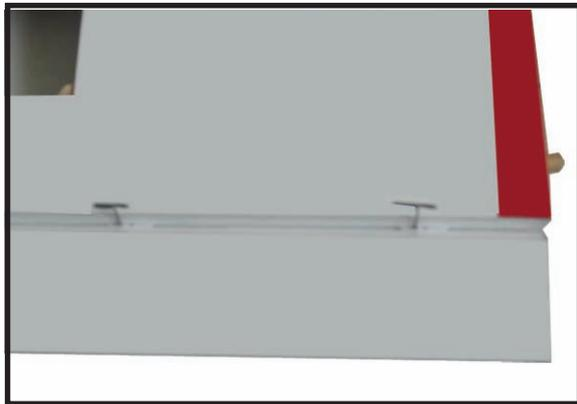
□ 4) Deflect the aileron and completely saturate each hinge with thin C/A glue. The aileron's front surface should lightly contact the wing during this procedure. Ideally, when the hinges are glued in place, a 1/64" gap or less will be maintained throughout the length of the aileron to the wing panel hinge line.
