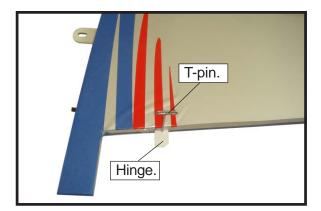
$\Box$  3) Slide the aileron on the wing panel until there is only a slight gap. The hinge is now centered on the wing panel and aileron. Remove the T-pins and snug the aileron against the wing panel. A gap of 1/64" or less should be maintained between the wing panel and aileron.
