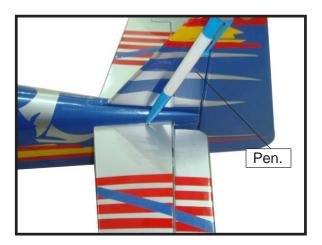
□ 4) Remove the stabilizer. Using a modeling knife, remove the covering from below the lines you drew.
