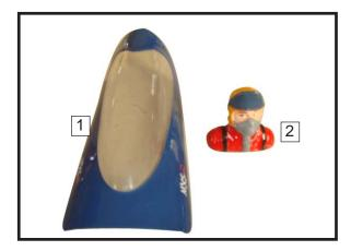
2) Position the pilot figure on the canopy floor as show. Locate the oval shaped on the canopy floor and remove the covering. Use epoxy to glue this into the base of the pilot figure, please see pictures as shown.
