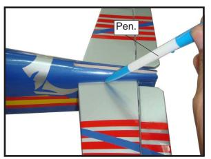
$\Box$  7) Remove the stabilizer. Using the lines you just drew as a guide, carefully remove the covering from between them using a modeling knife.
