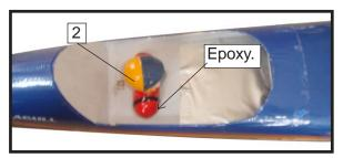
3) Position the canopy onto the fuselage. Trace around the canopy and onto the fuselage using a felt-tipped pen.
