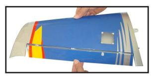
$\Box$  5) Turn the wing panel over and deflect the aileron in the opposite direction from the opposite side. Apply thin C/A glue to each hinge, making sure that the C/A penetrates into both the aileron and wing panel.
