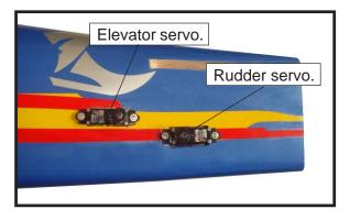
FUSELAGE SERVO ARM INSTALLATION.
