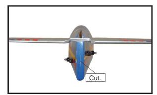
□ 2) Slide the vertical stabilizer into the slot in the top of the fuselage. The rear edge of the stabilizer should be flush with the rear edge of the fuselage and the lower rudder hinge should engage the precut hinge slot in the lower fuselage. The bottom edge of the stabilizer should also be firmly pushed against the top of the horizontal stabilizer.
