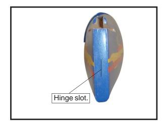
□ 6) With the stabilizer held firmly in place, use a pen and draw lines onto the stabilizer where it and the fuselage sides meet. Do this on both the right and left sides and top and bottom of the stabilizer.
