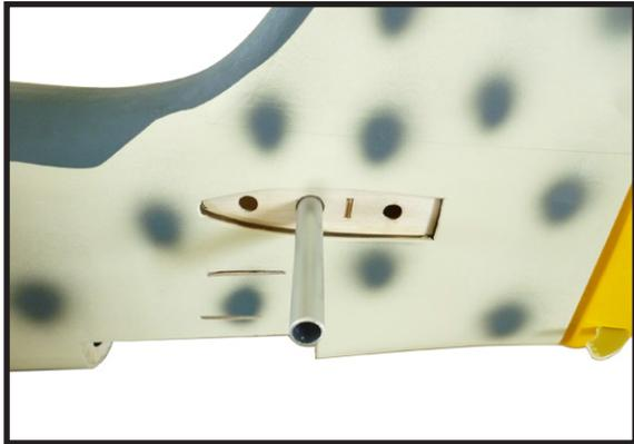
Use Epoxy Glue to glue the Horizontal Stabilizer to the fuselage.
