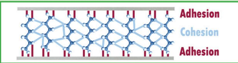
Epoxies produce greater strength across gaps because of the chemical reaction between adhesive molecules in the joint.
