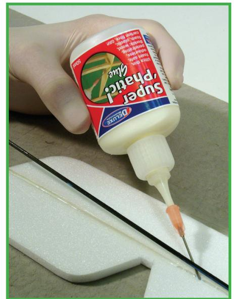
A modern low viscosity adhesive that can penetrate porous surfaces and has a low surface energy is a useful addition to the modellers armoury for foam and plastics.
